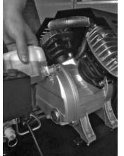
Always check the oil level in the pump before use. When filling, fill the oil from the oil breather hole until the oil reaches the red mark on the sight glass.
