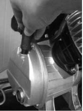
2. Check that the small hole in the top of the breather pipe is clear and then insert it into the oil filler hole.
