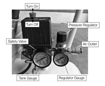
The pressure of the regulated outlet can be changed by turning the control knob. Rotate the knob clockwise to increase pressure and anti-clockwise to decrease.
